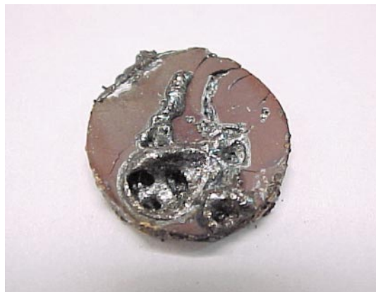
Fig. 1 Photograph of the product of an SHS reaction of \text{SrO}_2 , Fe and \text{Fe}_2\text{O}_3 in an applied field of 15 T. The disk has a diameter of 17 mm. The clear separation between metallic and non-metallic parts is typical of the products of hexaferrite reactions.
